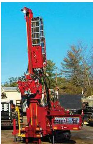
*Drill rig used to collect soil*
